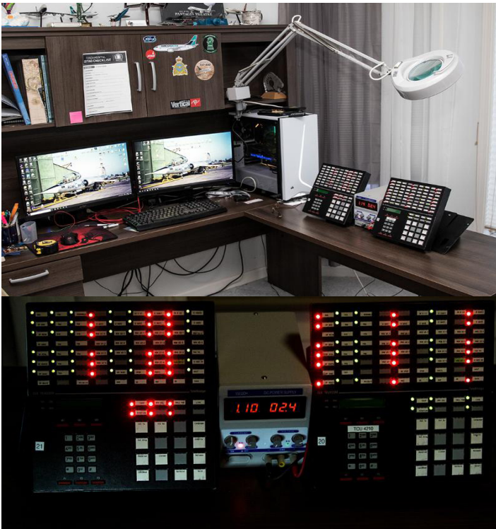
Panel lights from the radar console being worked on at Gary Watson's desk. All the wires had been cut so Gary rewired it for a new power supply . . . among other things. Gary Watson photo.
